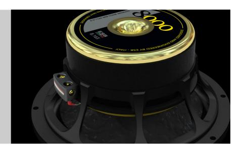
Y35 ferrite magnet motor is optimized with FEA simulation to ensure a perfectly symmetrical magnetic flux in both directions of cone's run. Motor metal parts are CNC machined from solid and refined material for maximum magnetic flux linearity and minimum magnetic loss. This reduces distortion at high power levels.
