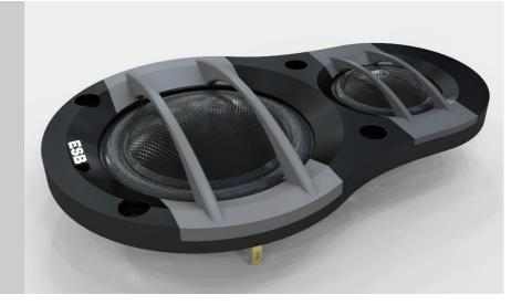
This special and exclusive component driver is a concept born way back in 70's, its aim is to concentrate medium and tweeter emissions in a single virtual point. This minimizes phase delays and irregularities at the crossover point.
